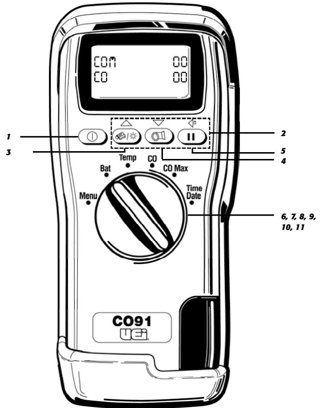
1. **Power Push-button** : Press "" button to switch the unit ON in fresh air outside the property about to be tested. This lets the meter auto calibrate its sensors properly.
